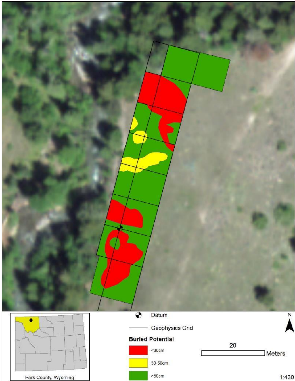
Figure 4.9. Buried potential map based on GPR data.
